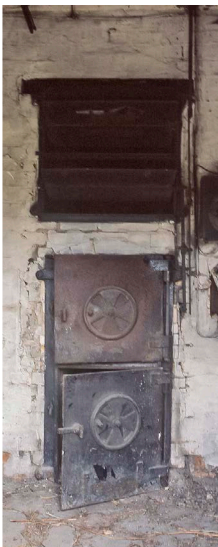
Above: Cirencester Brewery Maltings, Cricklade Street, Cirencester: H J H King patent furnace in south block. © Amber Patrick
