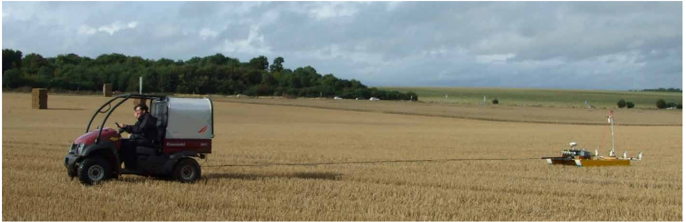
ATV-towed caesium magnetometer array at Boreland Farm in the WHS.
