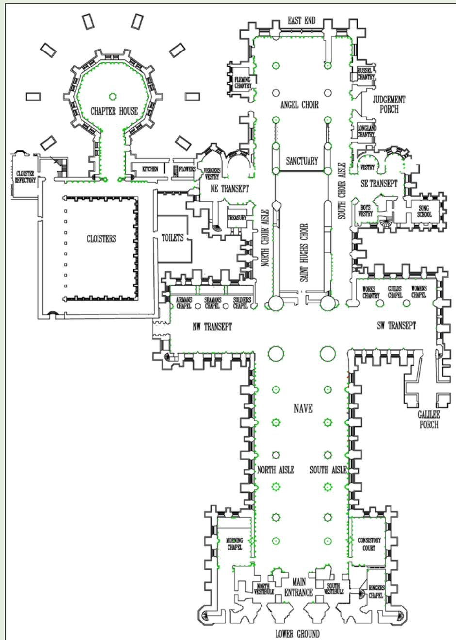
**Figure 35:** A ground floor plan of Lincoln Cathedral showing the location of Purbeck Marble elements.
