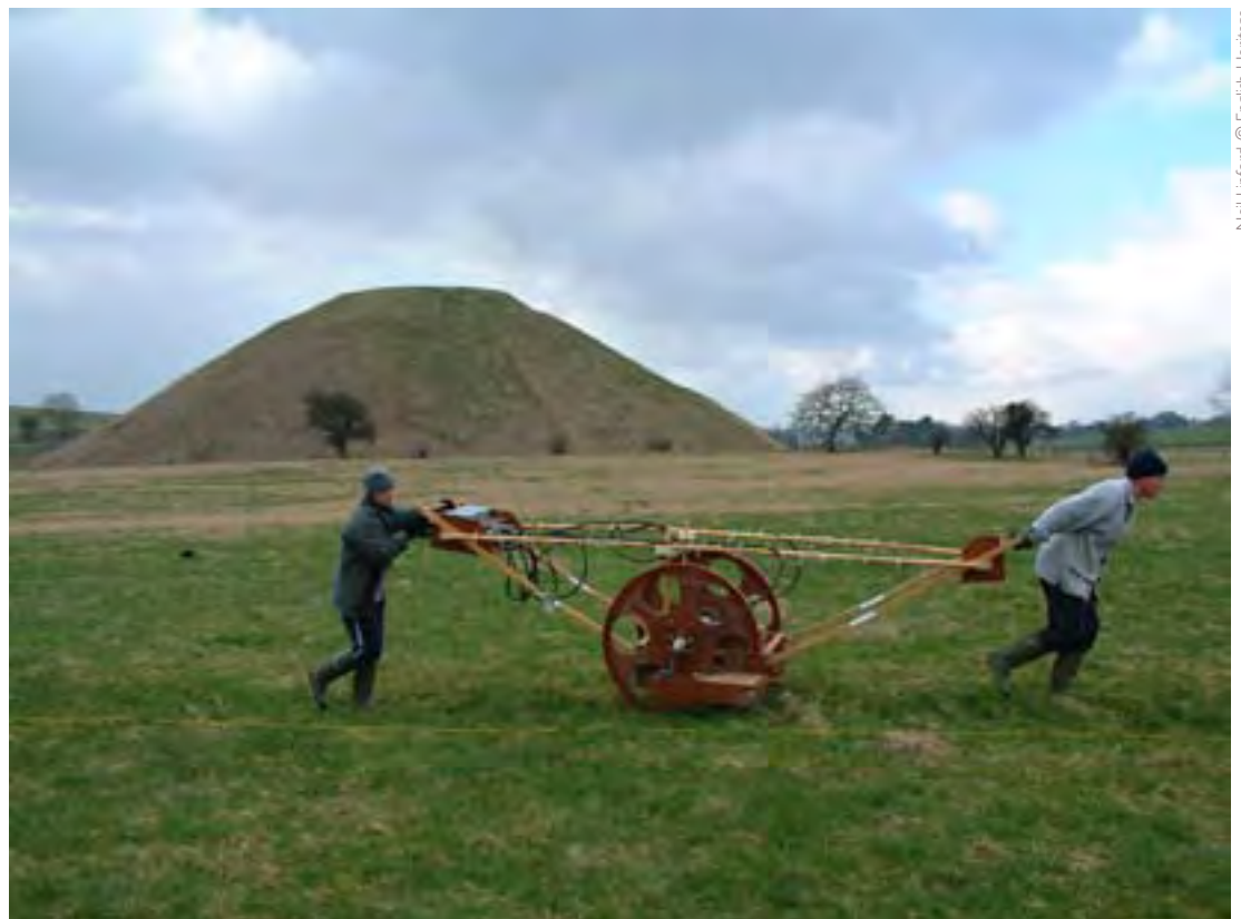
Geophysical survey in progress over the floodplain to the east of Silbury Hill using the EH cart mounted caesium magnetometer array
