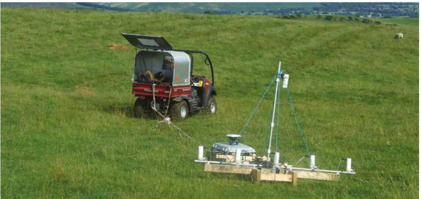
Development of the system, from hand-pushed to vehicle-towed. **Top left:** Hand Pushed Scintrex 4 sensor system, **top right:** Hand pushed system with GPS for "grid less" survey. **Bottom:** Vehicle towed system with GPS and 6 Geometrics sensors
