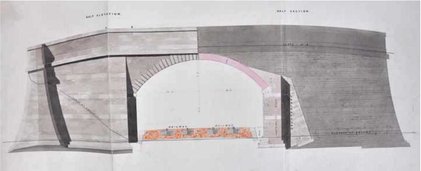
An original elevation drawing showing a typical North Midland Railway overbridge.
