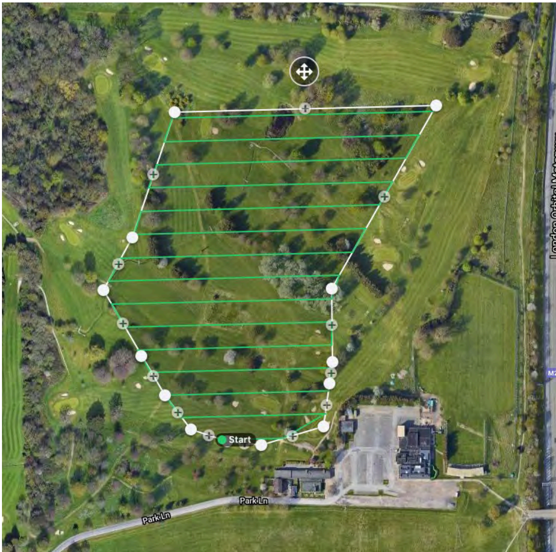
Figure 3 UAV pre-programmed mapping flight covering an area of 17 acres.
