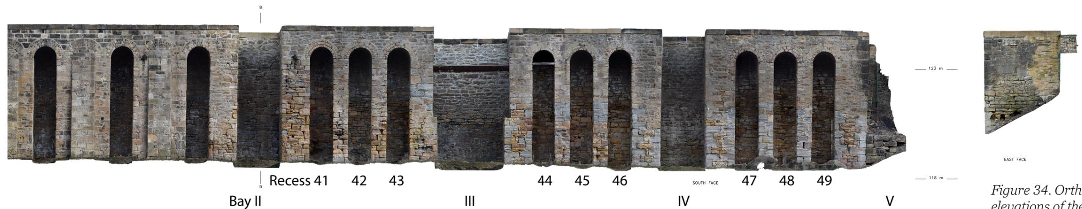
Figure 34. Orthophotographic elevations of the south face of the Coal Drops (recess 25 to end) and of the west face of bay V. From original survey drawings. [© Historic England].
