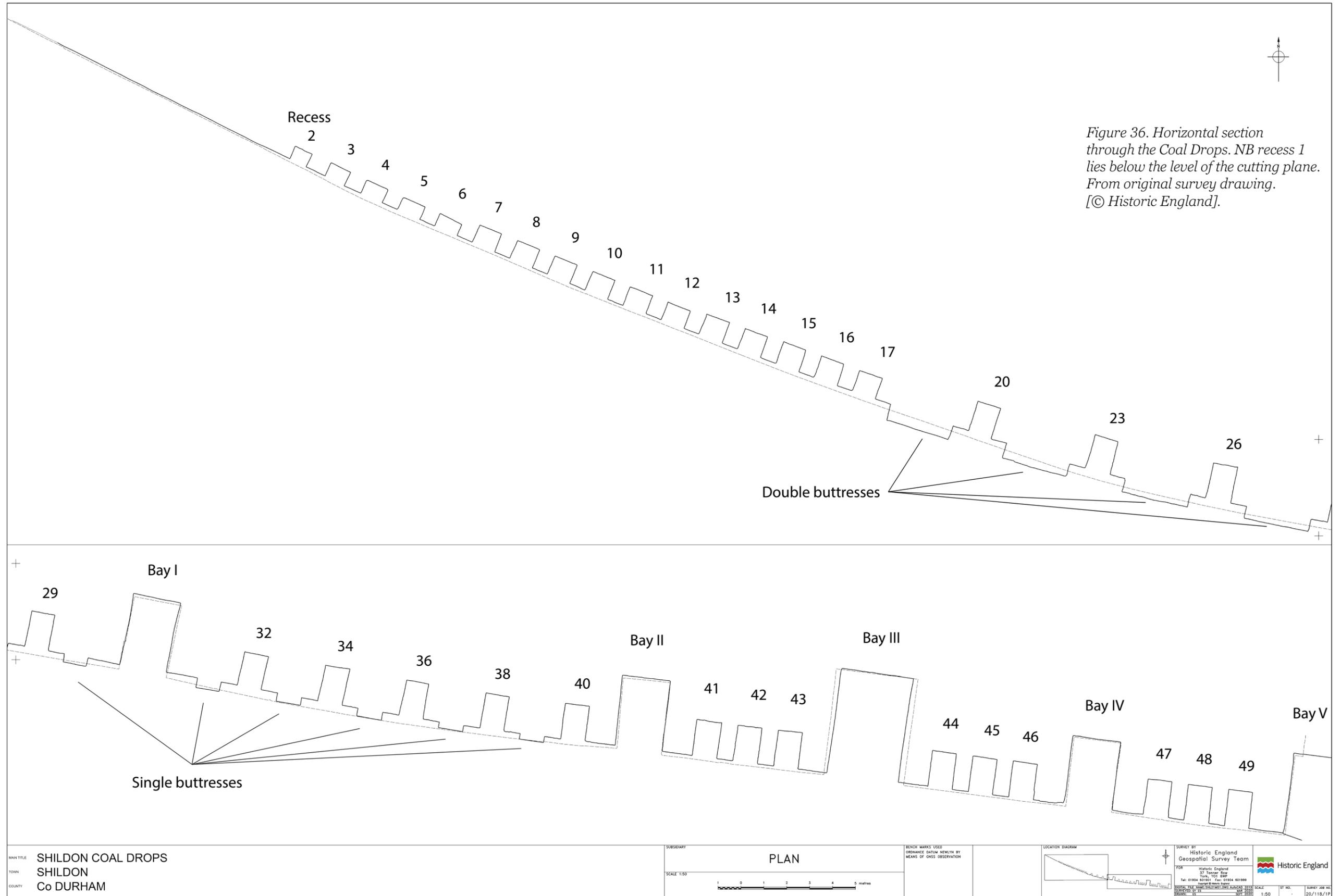
Figure 36. Horizontal section through the Coal Drops. NB recess 1 lies below the level of the cutting plane. From original survey drawing. [© Historic England].
