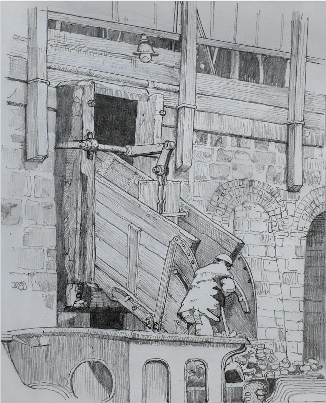
*Figure 18. Reconstruction drawing of a locomotive taking on coal using the hopper/chute mechanism, based on historic photographs especially Figure 7. [Allan Adams © Historic England].*
