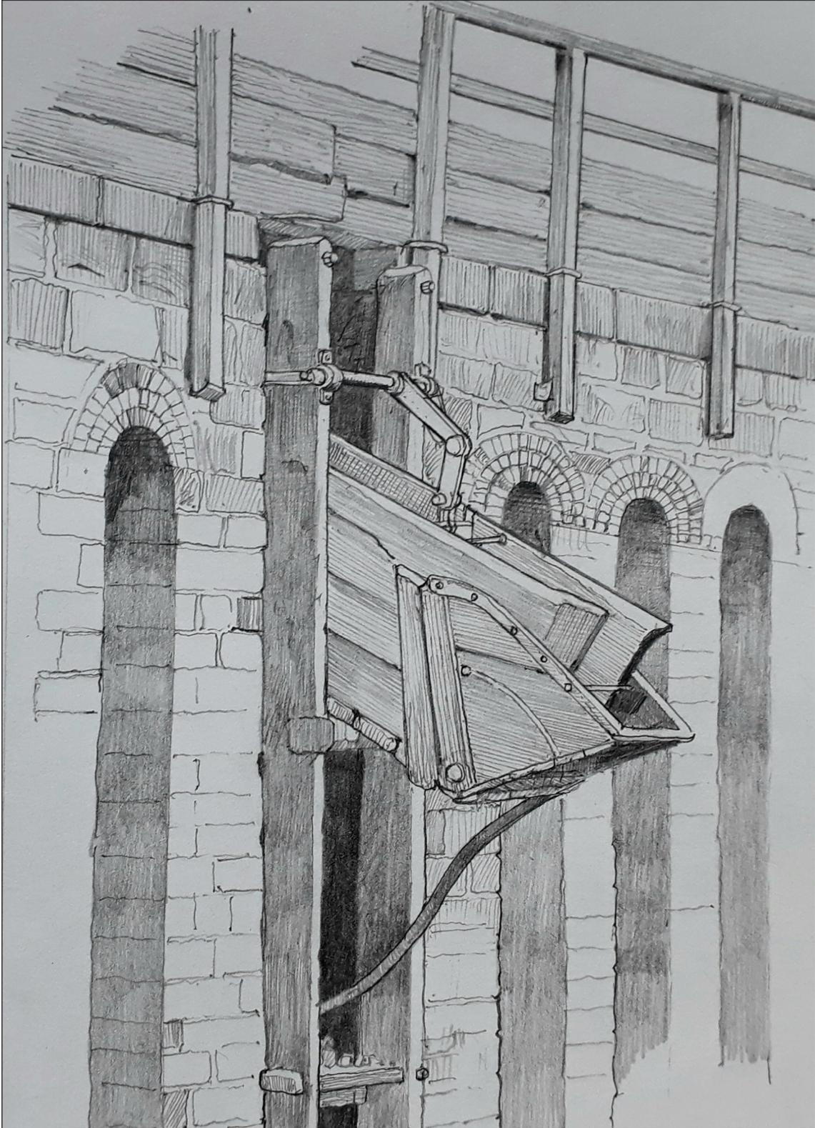
*Figure 17. Reconstruction drawing of the hopper/chute mechanism, based on historic photographs, especially Figure 7. [Allan Adams © Historic England].*
