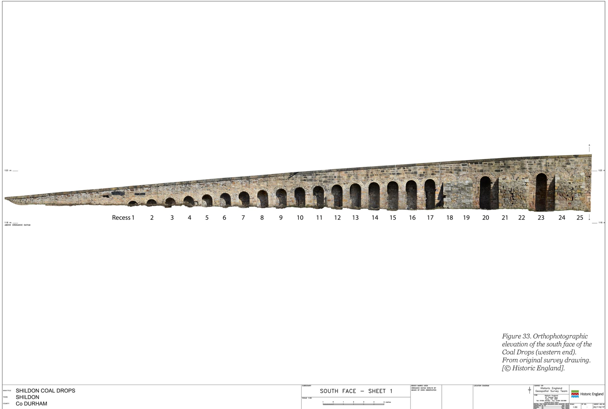
Figure 33. Orthophotographic elevation of the south face of the Coal Drops (western end). From original survey drawing. [© Historic England].
